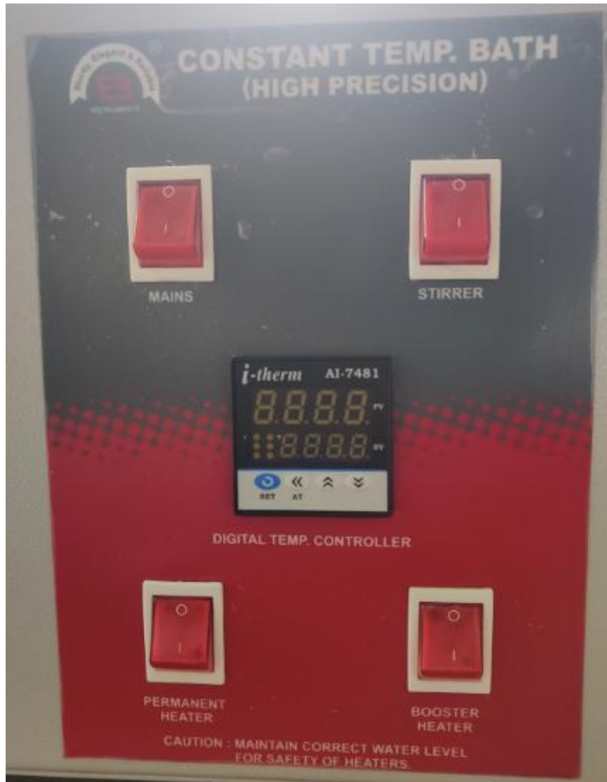
Figure 3 Control Panel & Digital controller
